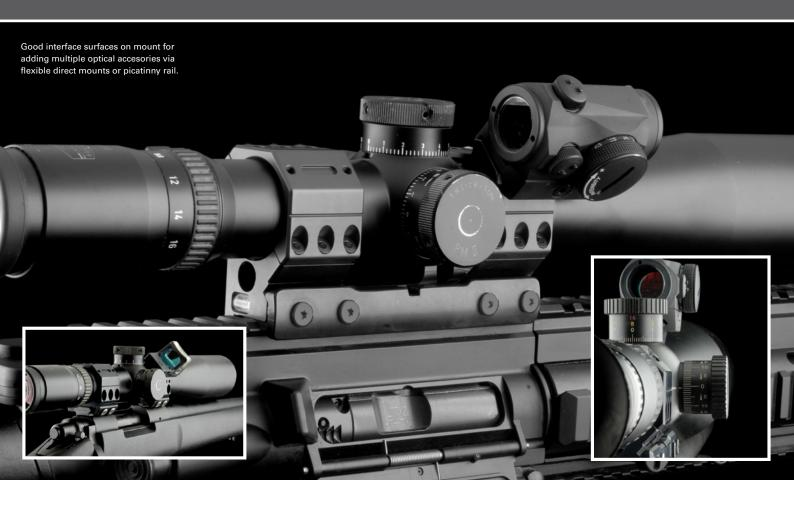
Extremely sturdy one-piece scopemount, with possibility to attach multiple optical accessories directly to the mount. Built-in level. 45 degree split of the rings gives better view of the turrets. 20MOA, 30MOA or customer specified tilt.
